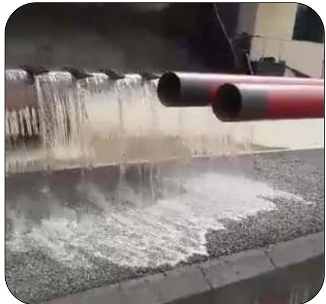
Fig 6 Water percolation demonstration through *Perviouscrete™*
